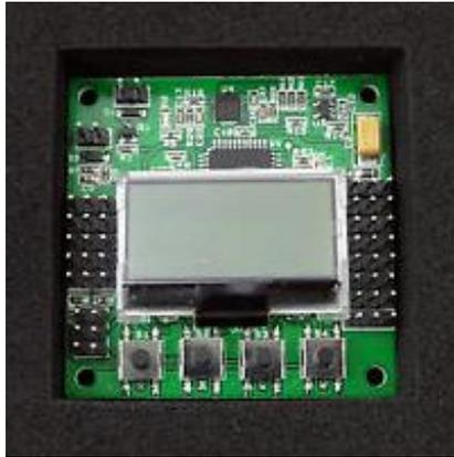
**STEP-1** Mount the FC on the frame with the LCD facing front and the buttons facing back.
