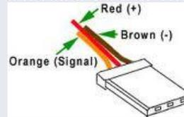
Ensure the negative (black or brown) is orientated so that it is on the pin that is nearest to the edge of the Flight Controller Board, so looking at the board the colour sequence will be Black, Red and Orange. The channels are connected as follows from the front of the board towards the push buttons: -
