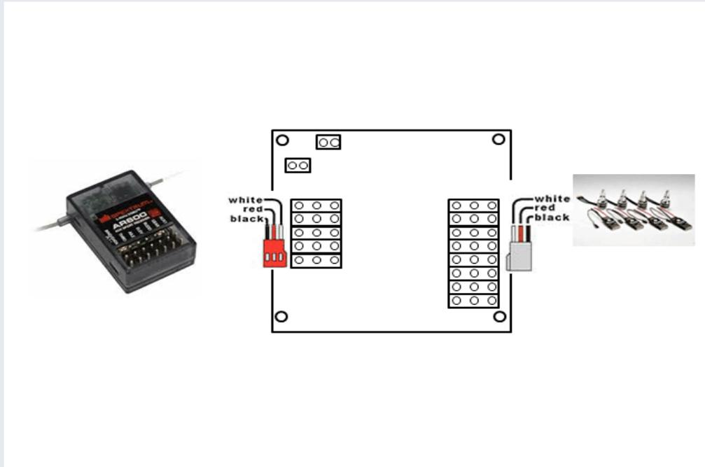
The Flight Controller Board must always have a source of +5v from an ESC, either one of the motors ESC or from a separate unit feeding the Receiver. If each ESC has a BEC (normal unless OPTO types) then it may be necessary to remove the power feed from the other ESC, usually by cutting the power line (RED) Cable on the other ESC.
